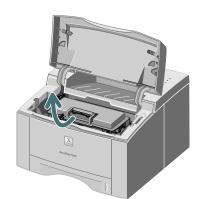
Open the top cover and remove the print cartridge. Once the print cartridge is removed from the printer, be careful not to expose it to heat or direct sunlight.
